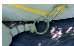
Metal clips to link booms.
