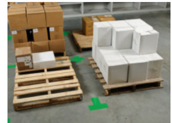
3. Colour-code material storage areas.
