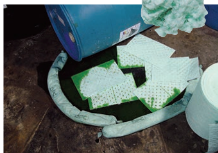
Fast containment of chemical spills.
