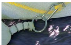
Metal clips to link booms.
